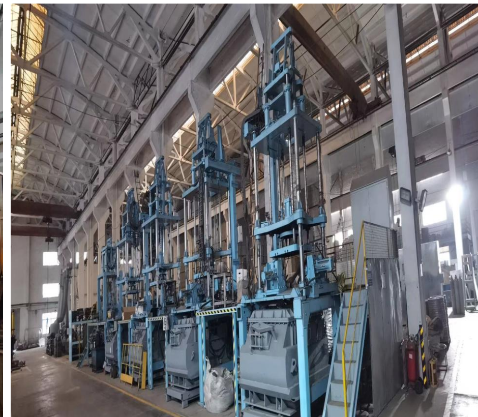
低压压铸区 Low pressure die-casting area
